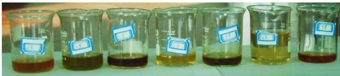
Fig. 1. The color of the extraction solution obtained by HPE. The conditions of HPE, from left to right: (1) 200 MPa holding 5 min, 0 MPa holding 5 min, 600 MPa holding 5 min, solvent is 50% ethanol; (2) pressure and holding time are same as 1, solvent is 70% ethanol; (3) 400 MPa holding 5 min, solvent is 70% ethanol; (4) 400 MPa holding 10 min, solvent is water; (5) 600 MPa holding 5 min, 0 MPa holding 5 min, 600 MPa holding 5 min, solvent is 70% ethanol; (6) 600 MPa holding 5 min, solvent is water; (7) 600 MPa holding 10 min, solvent is 50% ethanol.
